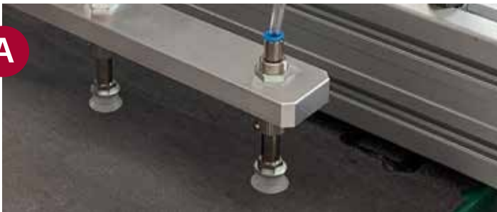
Sheet feeder with suction cups
