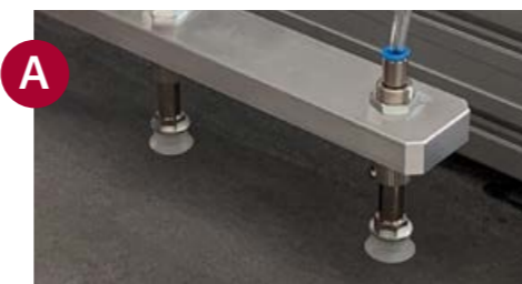
A Sistema a ventose Sheet feeder with suction cups
