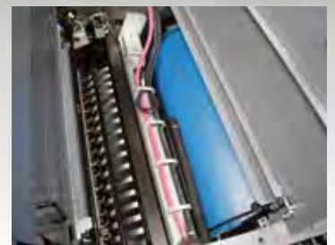
LED-UV curing unit over the convertible perfecting device
