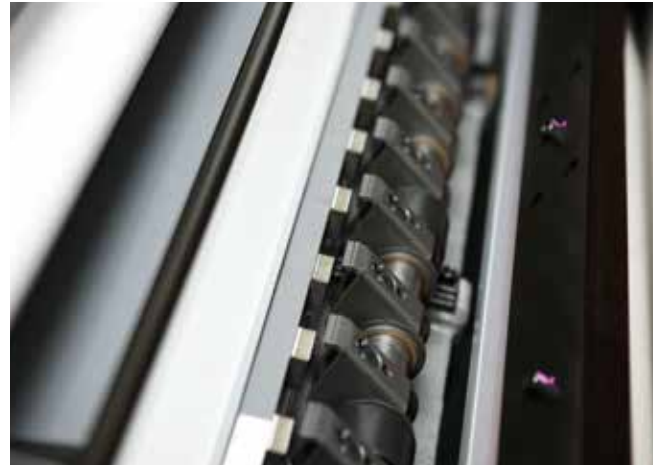
Double sprung gripper mechanism employing torsion bars
