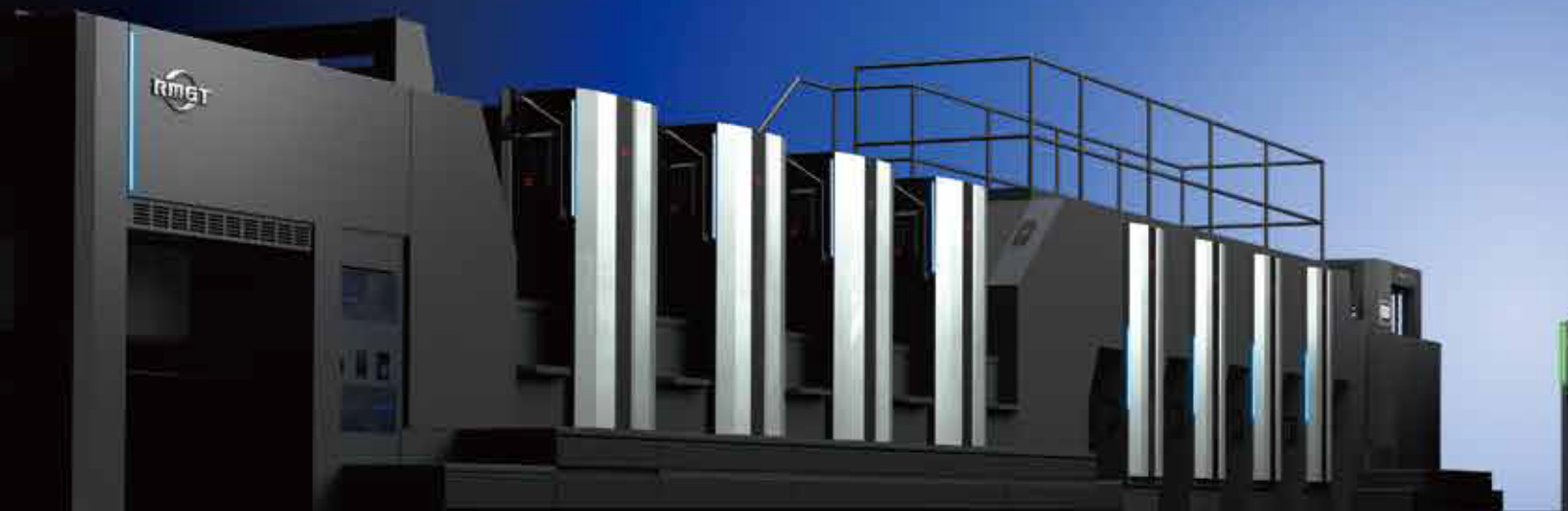
1060TP-8 (1060 mm Format 8-color Tandem Perfecter Offset Press)
