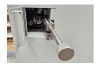
The PT interchangeable crease/perf die system makes for the fastest changeover between crease and perf dies. Run your greeting cards with a professional crease to prevent cracking and then quickly slide out the die and replace it with a perf die to run off easy tear coupons for the next customer. The rubber crash pad perfing system is an economical solution for partial perforating. Offer more to your customers without breaking the bank to purchase costly accessories and upgrades.
