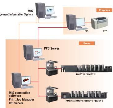
(Note) The IPC Server II is required to connect RMGT 10 or RMGT 11 to an MIS system.
